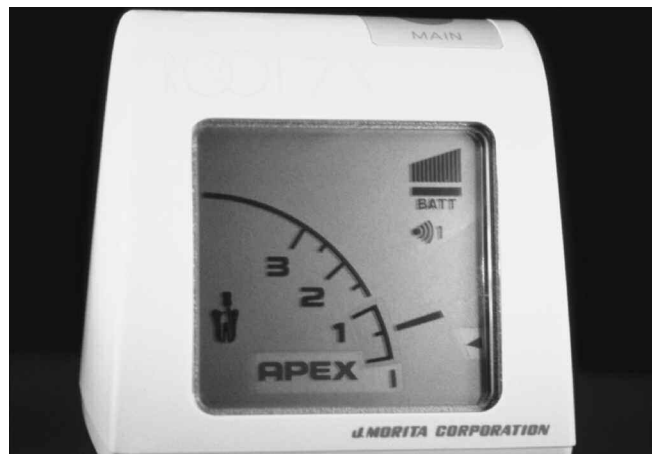
Figure 11b. The Root ZX has a large backlit screen, an easy to read digital read-out, and provides an accurate method for determining working length.
