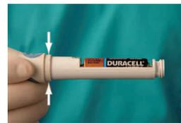
4. Confirm the placement of a high quality lithium battery and select the new Battery Housing Replacement Part. Before proceeding, turn the screw cap on the new part, in a counterclockwise direction as noted above. Also note the elevated male orientational tracks (see arrows).
