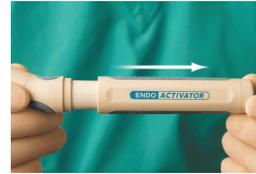
2. Rotate the screw cap counterclockwise to disengage and progressively remove the battery housing from the handpiece, then discard.
