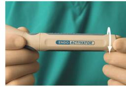
1. To remove the damaged battery housing, firmly grasp the contra-angled portion of the handpiece with one hand and begin turning the non-removable screw cap counterclockwise with the other hand.
