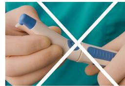
3. DO NOT grasp and forcefully rotate the battery housing! Cracking may result when excessive force is used to dislodge the male tracks from the female guide slots. *Only the battery access screw cap is rotated counterclockwise to disengage and progressively remove the battery housing as described above.*
